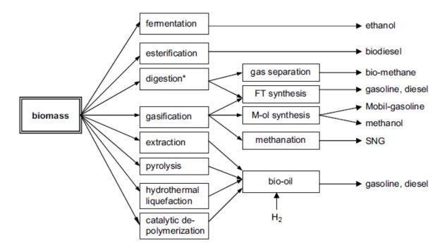
**Figure 1.1:** Main technological routes for the production of fuels from biomass as reported by Mudarov *et al* [10]. \*Anaerobic digestion to biogas followed by its reforming to syngas; M-ol – methanol; SNG – substitute NG
