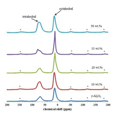
**Figure 5.6.** <sup>27</sup>Al MAS NMR spectra of  $\gamma$ -Al<sub>2</sub>O<sub>3</sub> and of Na<sub>2</sub>CO<sub>3</sub>/  $\gamma$ -Al<sub>2</sub>O<sub>3</sub> samples with different Na<sub>2</sub>CO<sub>3</sub> loadings. Asterisks denote spinning sidebands
