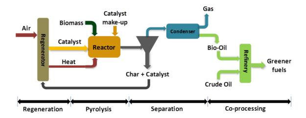
Figure 1.2: Conceptual scheme for green fuels from lignocellulosic biomass [16]
