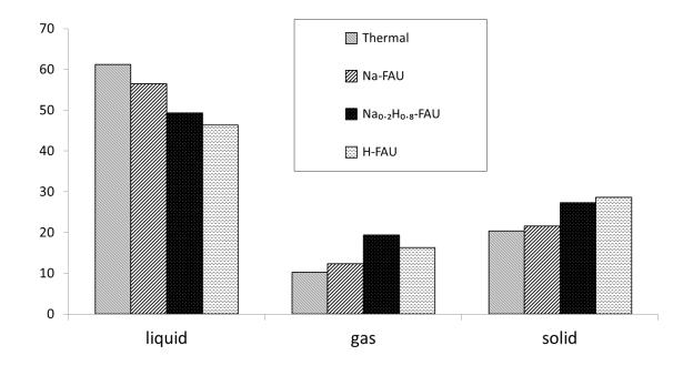
**Figure 3.4.** Product yields in catalytic and non-catalytic experiments
