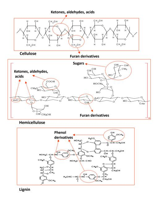
**Figure 3.2.** Chemical structure of cellulose, hemicellulose, lignin and the correlation to their products found in bio-oil
