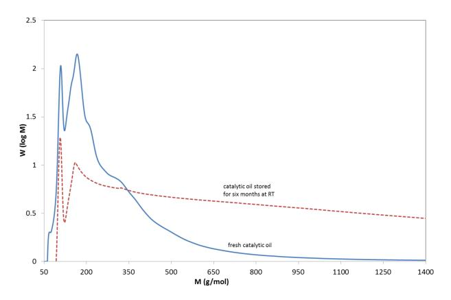
**Figure 4.1.** Molecular weight distribution of the fresh and old catalytic bio-oils analysed by GPC
