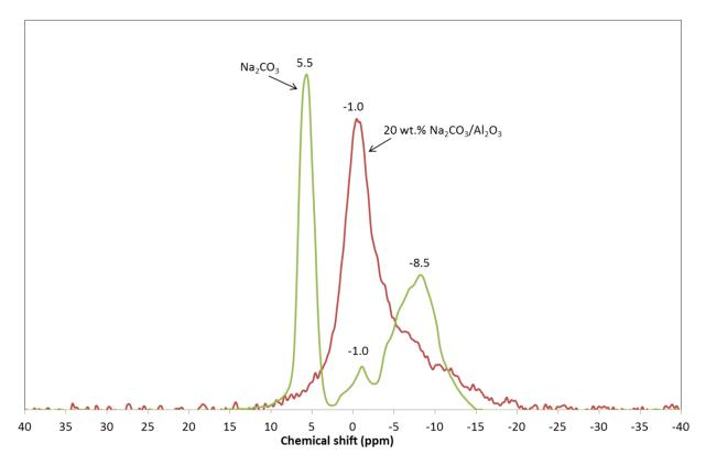
Figure 4.4. <sup>23</sup>Na MAS NMR spectra of pure Na<sub>2</sub>CO<sub>3</sub> and of the catalyst sample
