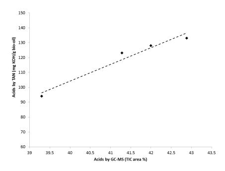
**Figure 3.5.** Correlation of TAN with total amount of acids in bio-oil; Measurement error of TAN analysis calculated to be 1.47% based on 95% confidence level
