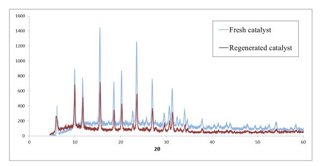
**Figure 3.8.** XRD analyses of fresh and regenerated catalysts
