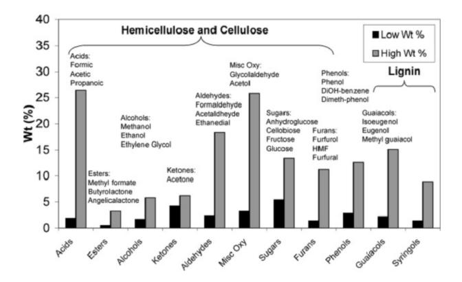
**Figure 1.3:** Chemical composition of bio-oils according to Milne *et al.* [17]. The graph also shows the most abundant molecules of each of the components and the biomass fraction from which the components were derived. The concentration of a certain group of compounds in bio-oil can fluctuate between the low wt.% and high wt.%
