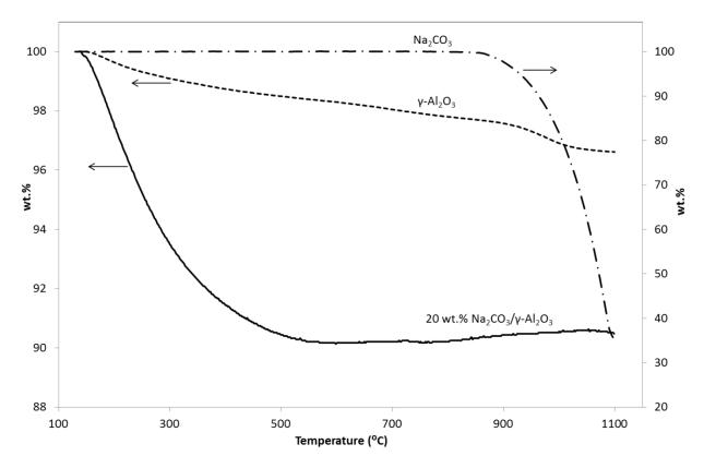
Figure 4.4. TGA analyses of the catalyst and its components
