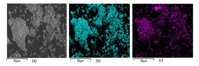
**Figure 4.2.** (a) SEM photograph, with EDX corresponding to (b) Al mapping and (c) Na mapping of the 20 wt.%  $Na_2CO_3/\gamma$ -Al<sub>2</sub>O<sub>3</sub> catalyst
