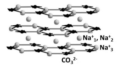
**Figure 5.4.** The crystal structure of Na<sub>2</sub>CO<sub>3</sub> showing positions of sodium cations and carbonate anions according to Arakcheeva and Chapuis [21]
