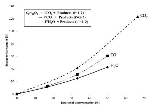
**Figure 3.3.** Efficiency of different oxygen removal routes, calculated using Dulong formula\*  $^*$ HHV (MJ/kg) = (0.3388\*[C])+(1.442\*([H] -[O]/8))
