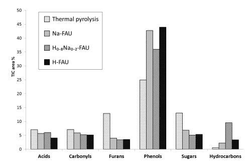
**Figure 3.6.** Distribution of chemical groups in bio-oils obtained from catalytic and non-catalytic experiments
