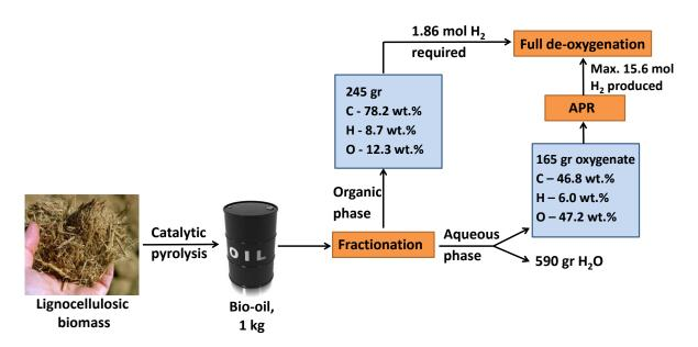
Figure 7.1. Estimation of hydrogen economic in bio-refinery of lignocellulosic biomass
