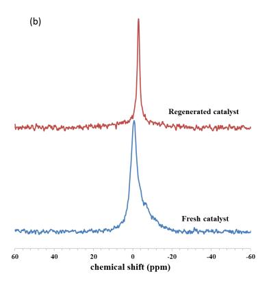
**Figure 5.7.** Comparison of properties of fresh and regenerated catalysts, shown by (a) XRD and (b) <sup>23</sup>Na MAS NMR analyses
