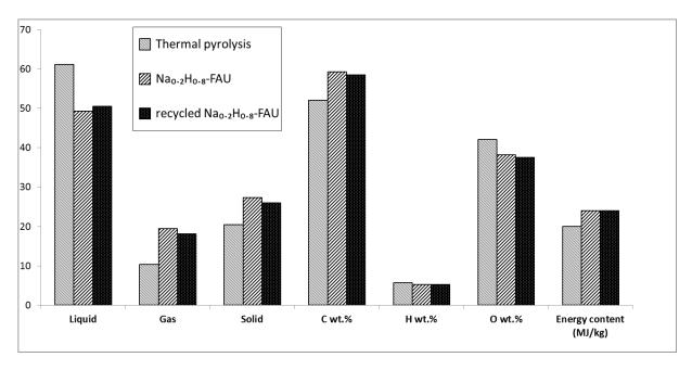
Figure 3.9. Comparing catalytic activity of fresh and recycled catalysts
