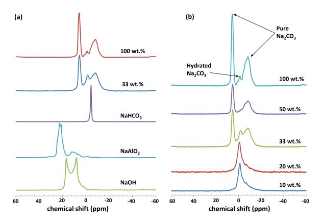
**Figure 5.3.** <sup>23</sup>Na MAS NMR spectra of (a) pure Na<sub>2</sub>CO<sub>3</sub>, 33 wt.% Na<sub>2</sub>CO<sub>3</sub>/  $\gamma$ -Al<sub>2</sub>O<sub>3</sub> and several sodium-containing candidates and (b) Na<sub>2</sub>CO<sub>3</sub>/  $\gamma$ -Al<sub>2</sub>O<sub>3</sub> with different mass concentrations of Na<sub>2</sub>CO<sub>3</sub>
