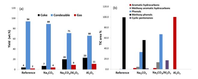
**Figure 6.3.** The effect of different catalysts to: (a) yields of coke, condensable, gas products, wt.% and (b) TIC area % of different groups in the condensable fraction. Reaction conditions: 500 °C, 2 s, 1 g of VA and 1 g of catalyst.
