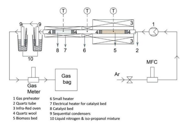
**Figure 2.1.** Schematic drawing of the fast pyrolysis experimental set-up
