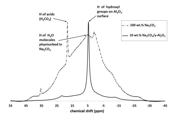
**Figure 5.5.** Comparison between <sup>1</sup>H MAS NMR spectra of 10% Na<sub>2</sub>CO<sub>3</sub>/γ-Al<sub>2</sub>O<sub>3</sub> and pure Na<sub>2</sub>CO<sub>3</sub> samples
