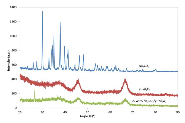
Figure 4.3. Comparison of XRD analyses of the catalyst and its two components
