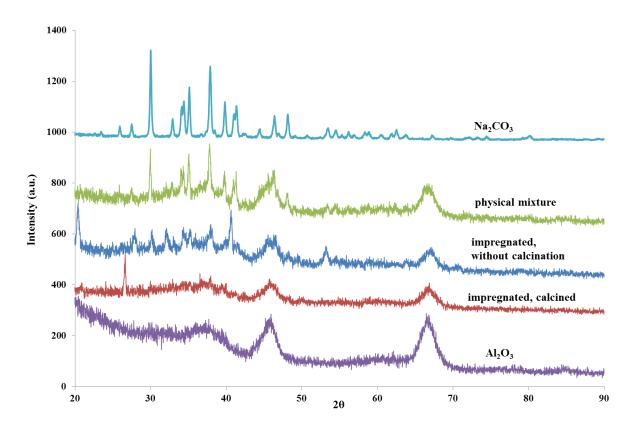
**Figure 5.1.** Comparison of different sodium carbonate dispersion shown by XRD diffractograms
