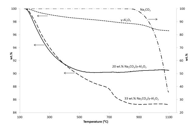
Figure 5.2. TGA analyses of the catalysts
