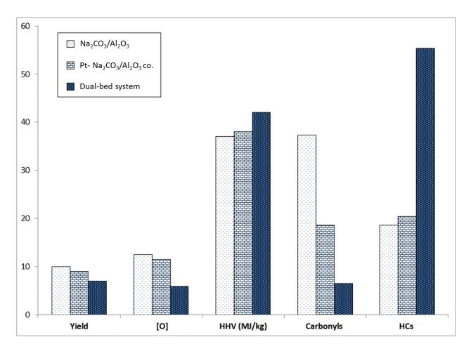
Figure 7.3. Comparison of single bed with dual bed towards bio mass hydro-pyrolysis
