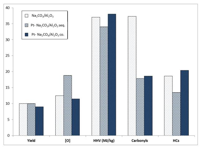
**Figure 7.2.** Comparison between two catalysts prepared by sequential impregnation and coimpregnation in biomass hydro-pyrolysis.
