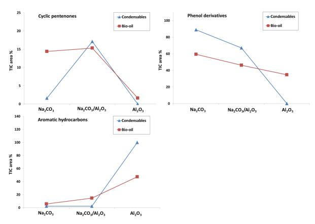
**Figure 6.7.** The change in composition of bio-oil from biomass pyrolysis and condensable (liquid) phase from VA conversion over different catalytic materials
