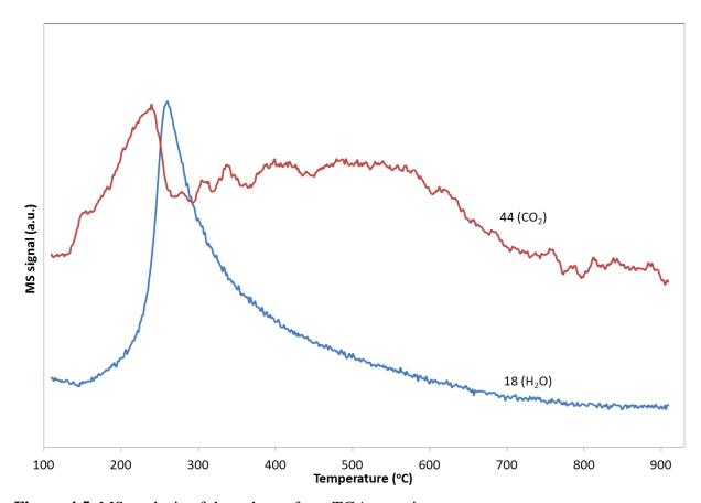
Figure 4.5. MS analysis of the exhaust from TGA experiment
